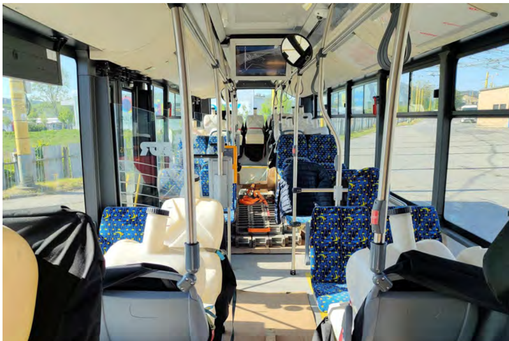
An interior view of No. 801 during the second stage of homologation, with a simulated load. [DPMP, a.s. - Juraj Handzuš]
