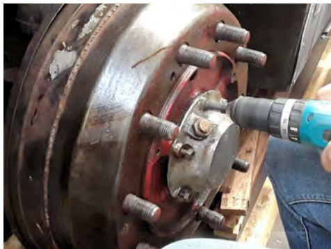
Cardiff 243's aluminium hub cover being unmovable, three of the six studs had to be drilled out. [Keith Walker]
