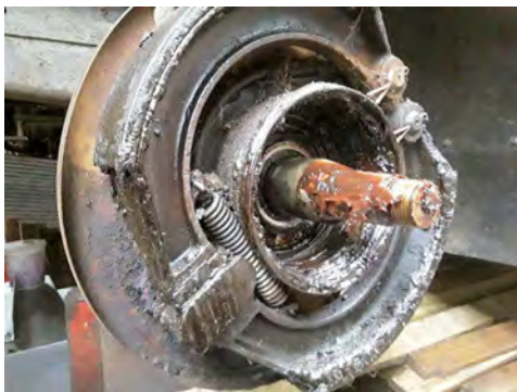
With the hub cover and the brake drum off and the hub seal having collapsed, a large coating of grease was applied, covering the brake shoes and assembly. [Keith Walker]
